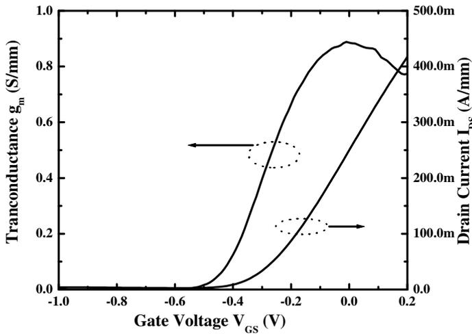
Fig. 5. Transfer characteristic of a  $0.25 \times 2 \times 50 \mu\text{m}^2$  composite channel HEMT.
