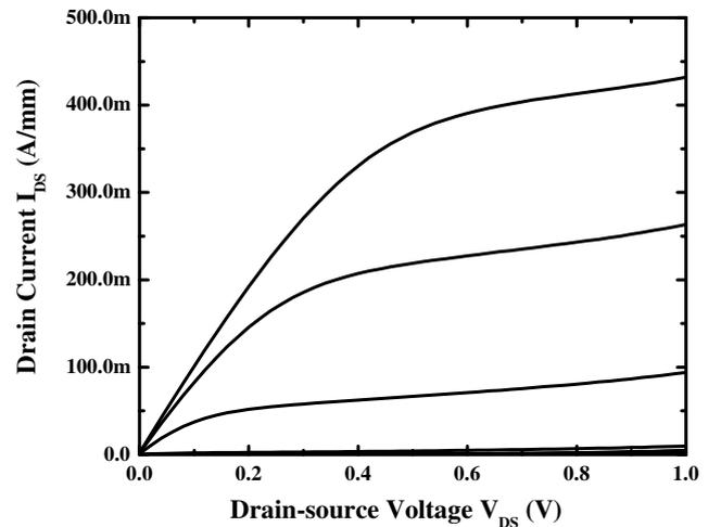
Fig. 4. DC I-V characteristic of a  $0.25 \mu\text{m} \times 2 \times 50 \mu\text{m}^2$  composite channel HEMT.
