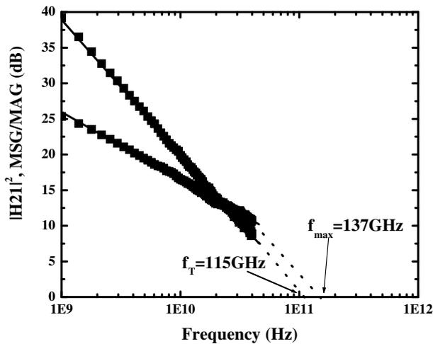
Fig. 6. Current gain and maximum stable/available gain characteristics of a typical  $0.25 \mu\text{m} \times 2 \times 50 \mu\text{m}^2$  composite channel HEMT.
