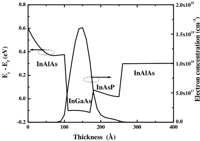
Fig. 2. Equilibrium conduction band diagram and electron distribution in composite channel HEMTs by solving Poisson and Schrodinger equation (thickness starts from barrier layer).
