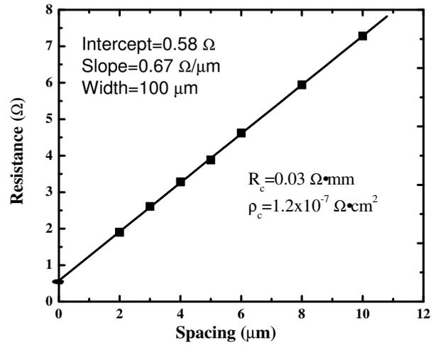
Fig. 3. Dependence of contact resistance on the spacing for TLM measurement.
